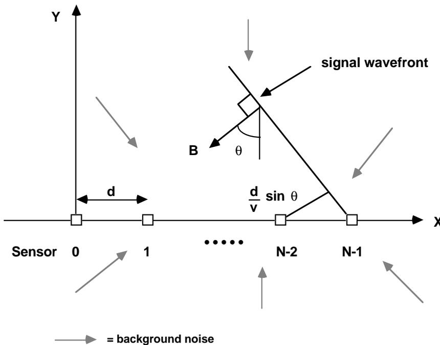
Figure 15.3 Line Array of Equally Spaced Hydrophones
