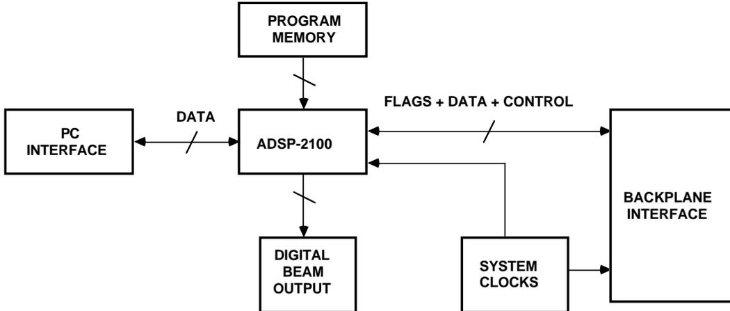
Figure 15.8 Master Module Block Diagram
