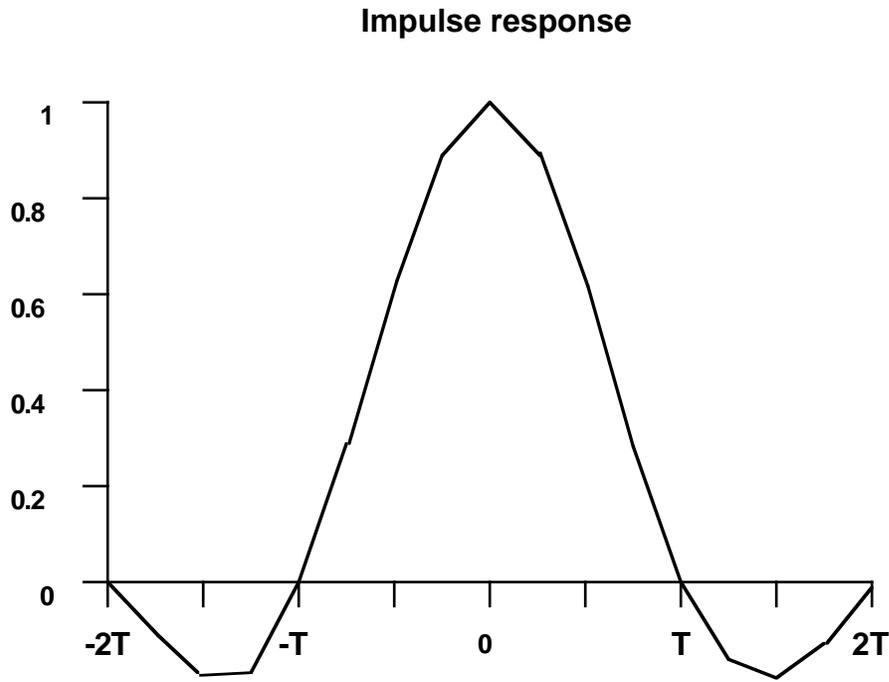
**Figure 2.8 Raised Cosine Pulse Shaping Filter,  $\alpha=0.25$**
