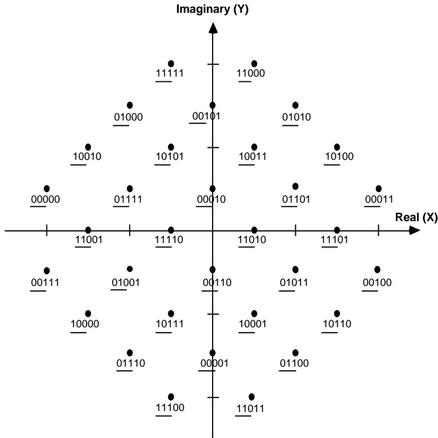
**Figure 2.14 Signal Constellation Showing Convolutional Encoder Output**
