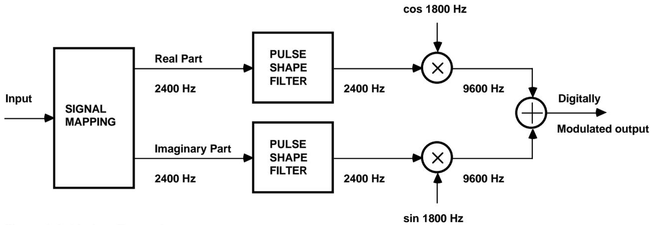
Figure 2.9 Modem Transmitter
